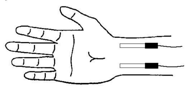
The figure illustrates the placement of two electrodes on the same wrist. It is easier to place the electrodes if you first place the strap around the wrist and then insert the electrodes under the strap.
