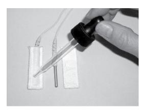
**Step 2:** Place the cotton sleeves over the electrodes. A dropper bottle is a handy way to wet the cotton and to keep the covers damp during use.
