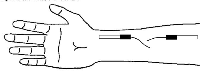
This figure illustrates the placment of the two electrodes on the same forearm and wrist. Position probes about 6" apart on the same Radial Artery.
